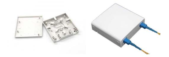
2 port mini odf indoor terminal applied in the FTTX network to connect the drop cable and optical devices through fibre port. VTB20 covers the capacity of 1 core, 2 cores and 4 cores and supports splicing, mechanical connection and FMC, wall mounted installation
